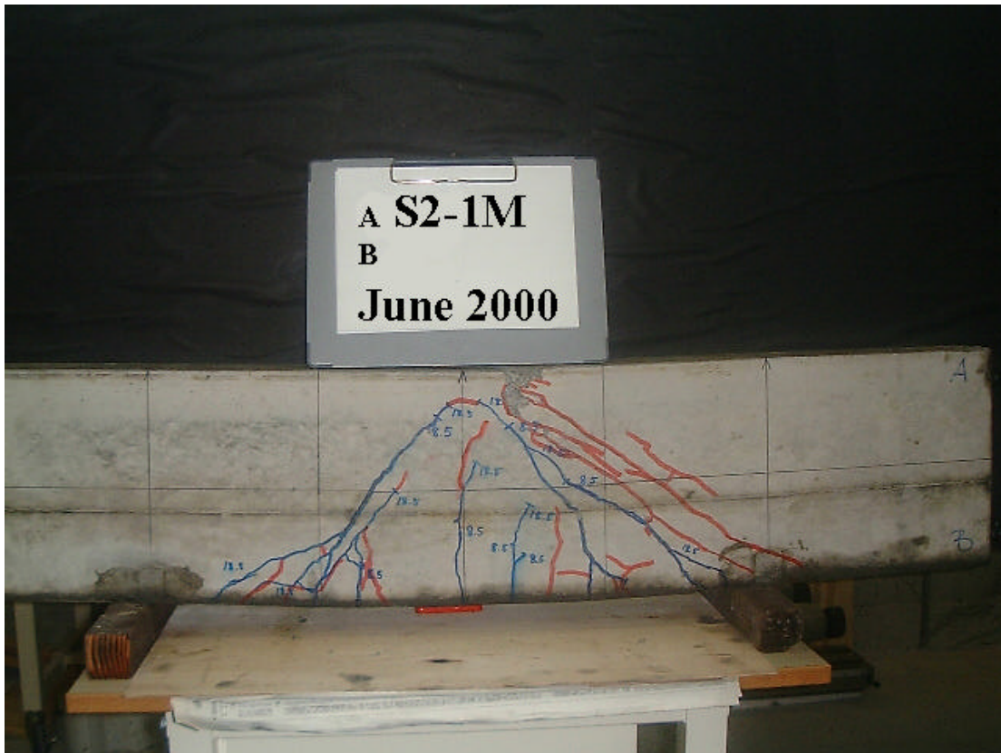
Fig. 5-31 Crack pattern of experimental result
