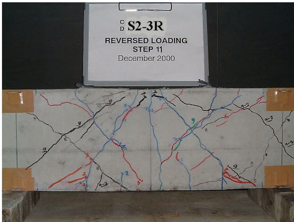
Fig. 5-16 Crack Pattern of specimen S2-3R under reversed loading
