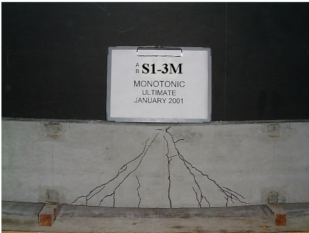
Fig. 5-6 Crack pattern of specimen S1-3M under monotonic loading
