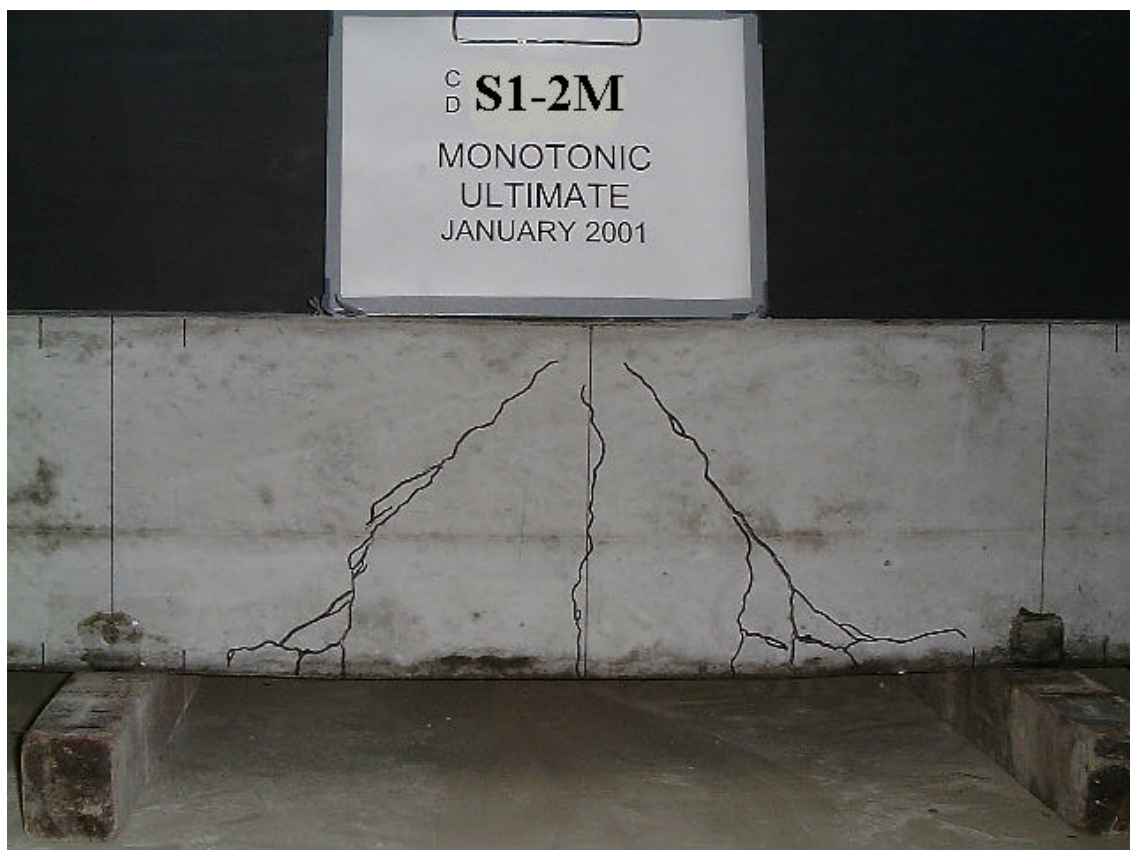
Fig. 5-27 Crack pattern of experimental result.
