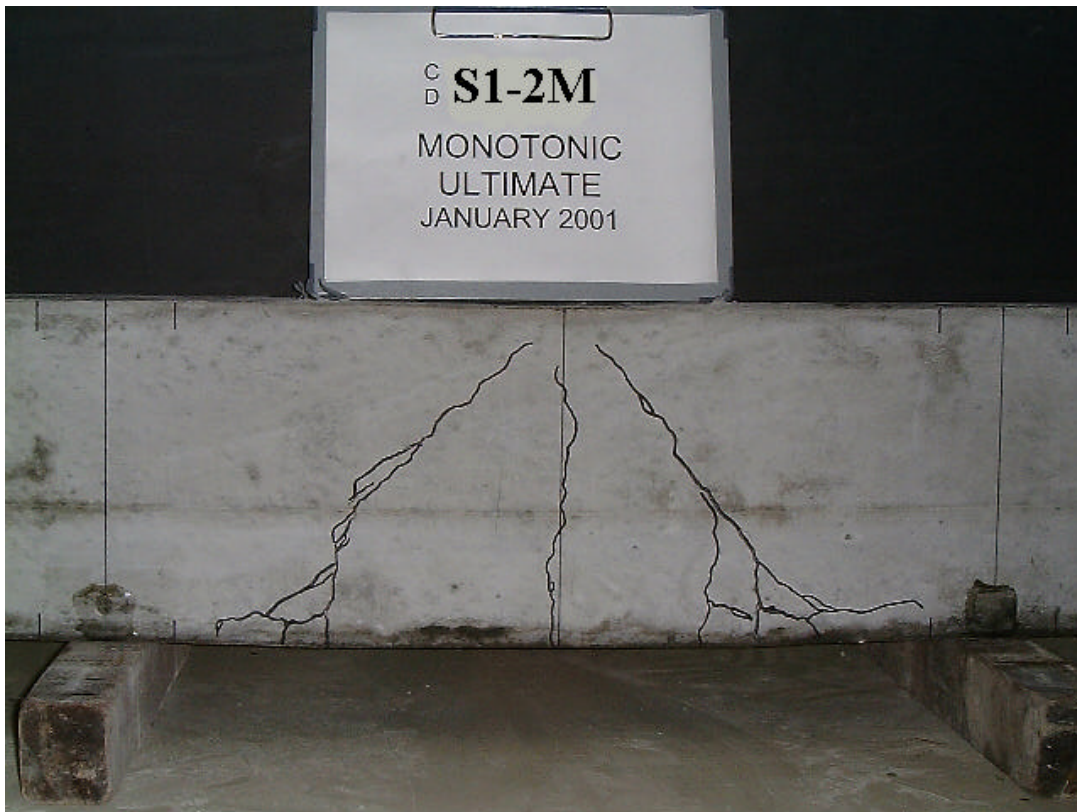
Fig. 5-4 Crack pattern of specimen S1-2M under monotonic loading
