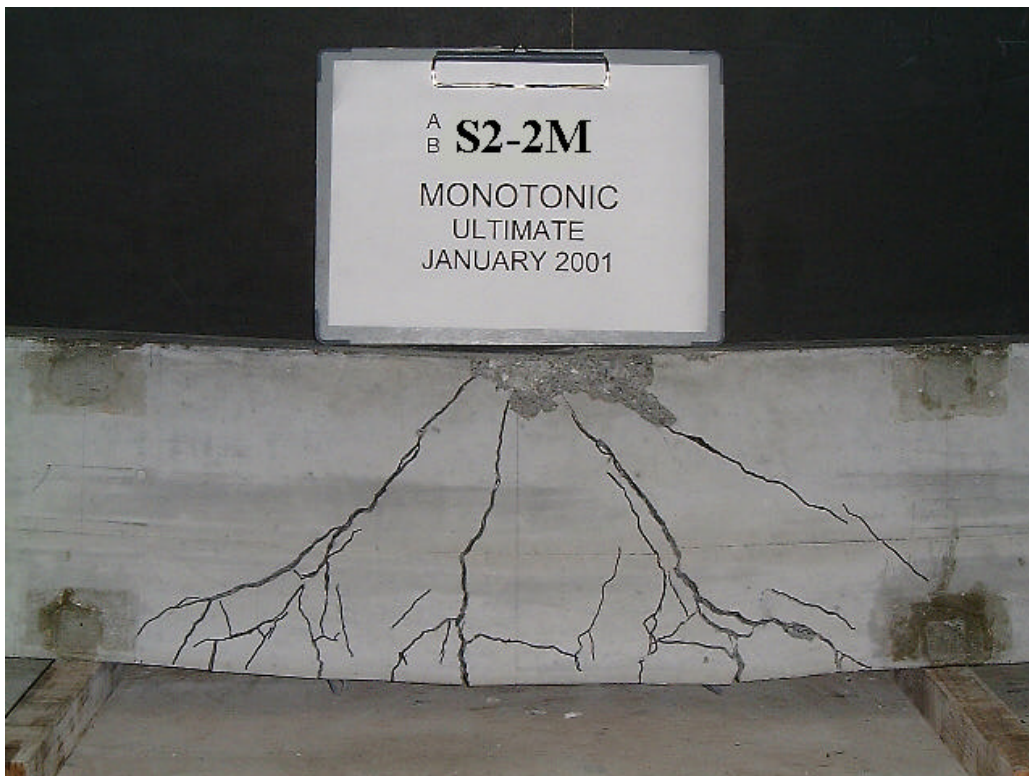
Fig. 5-10 Crack pattern of specimen S2-2M under monotonic loading
