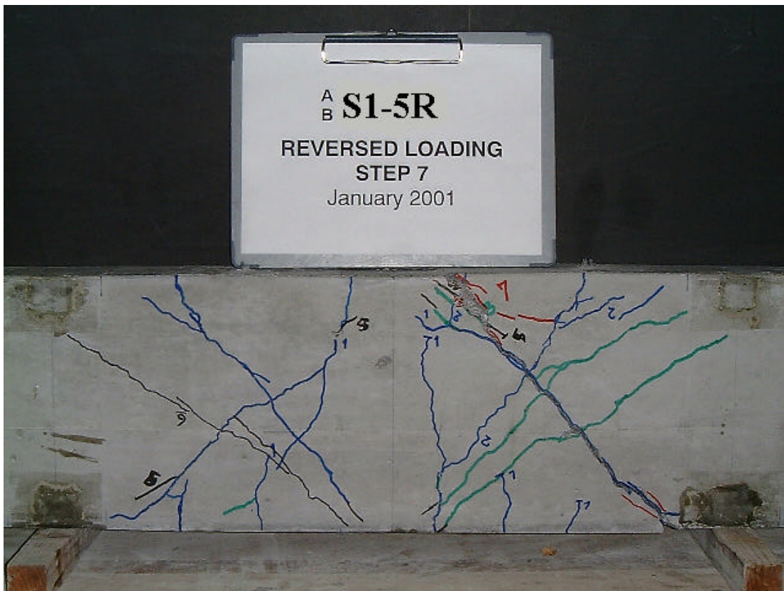
Fig. 5-14 Crack Pattern of specimen S1-5R under reversed loading
