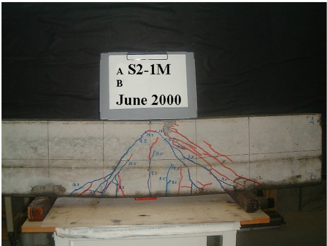
Fig. 5-8 Crack pattern of specimen S2-1M under monotonic loading
