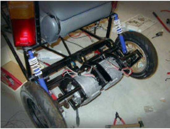
Figure 10 Rear Suspension and Motor Mount
