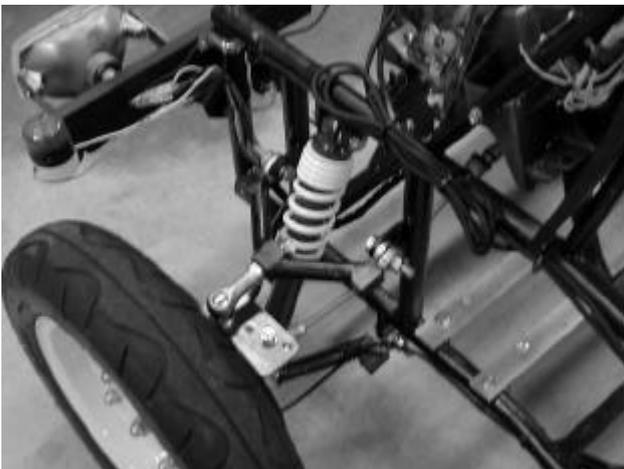
**Figure 7 Front Suspension System (With a Tire)**
