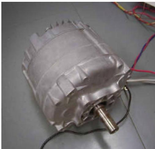
**Figure 3 Honda In-wheel Motor**
