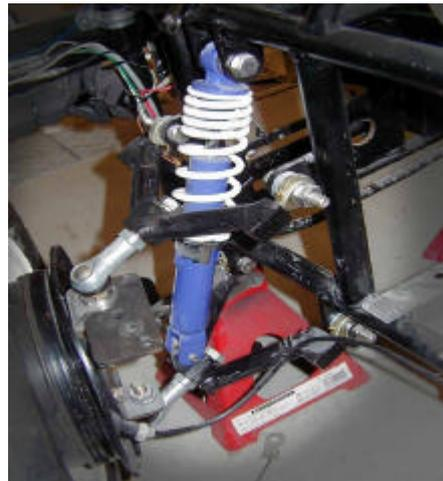
**Figure 8 Front Suspension System (Closer View)**
