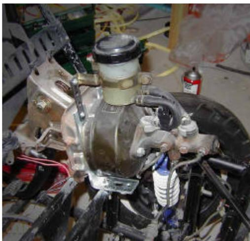
**Figure 16 Brake Cylinder for Pressure Amplifier**
