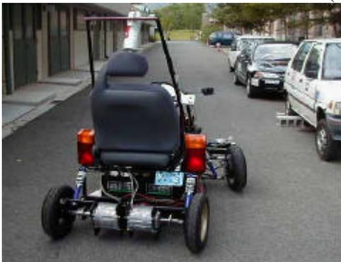
Figure 18 Hand-Made Small-Sized Electric Vehicle (Back View)
