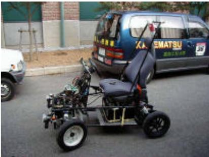
Figure 17 Hand-Made Small-Sized Electric Vehicle (Side View)
