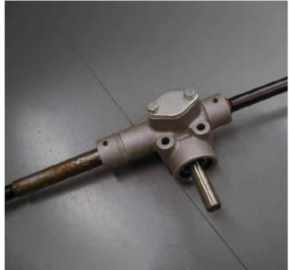
**Figure 9 Gear Box of Rack and Pinion Type**
