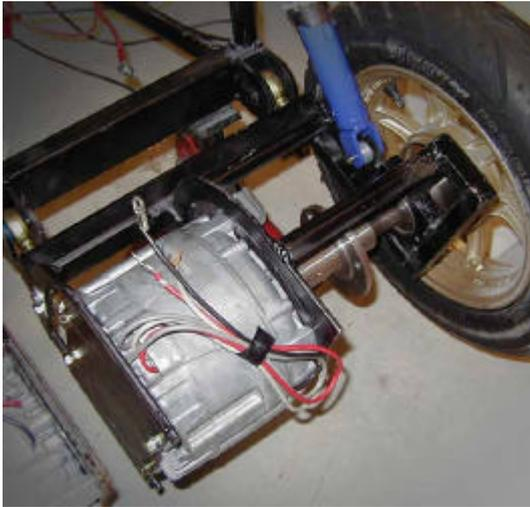
Figure 11 Rear Suspension and Motor Mount (Closer View)
