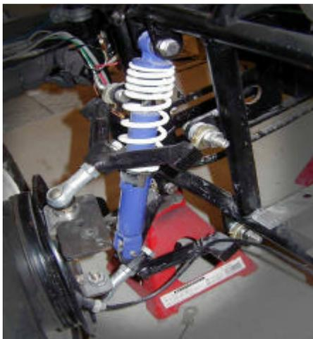
**Figure 8 Front Suspension System (Closer View)**
