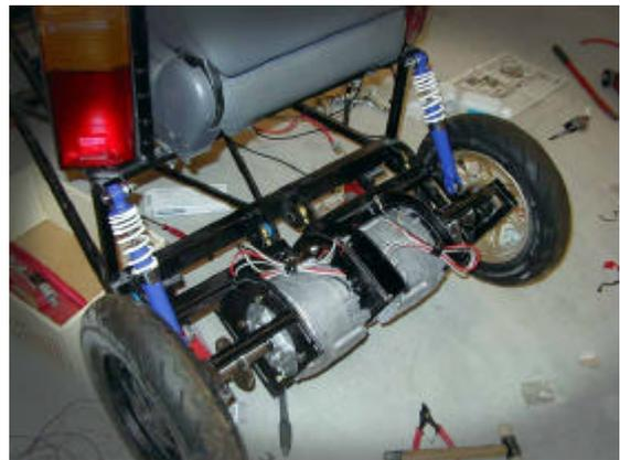
**Figure 10 Rear Suspension and Motor Mount**
