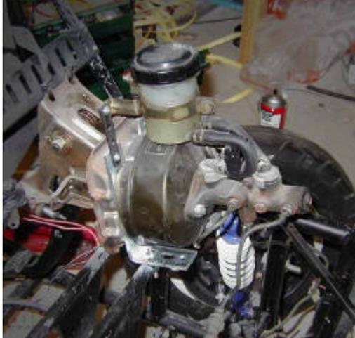
Figure 16 Brake Cylinder for Pressure Amplifier
