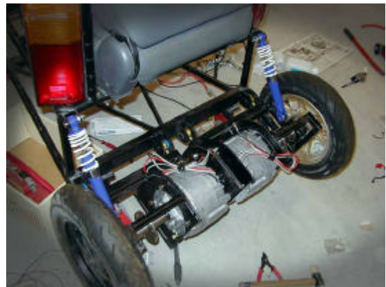
Figure 10 Rear Suspension and Motor Mount
