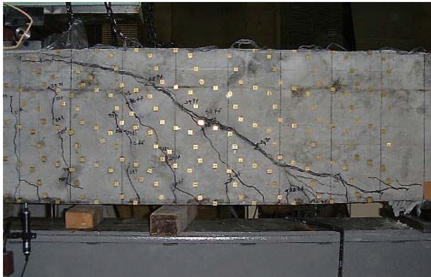
Figure.3_8: Shear Failure of Beam 3.
