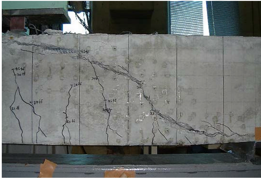
Figure.3_11: Shear Failure of Beam 4.
