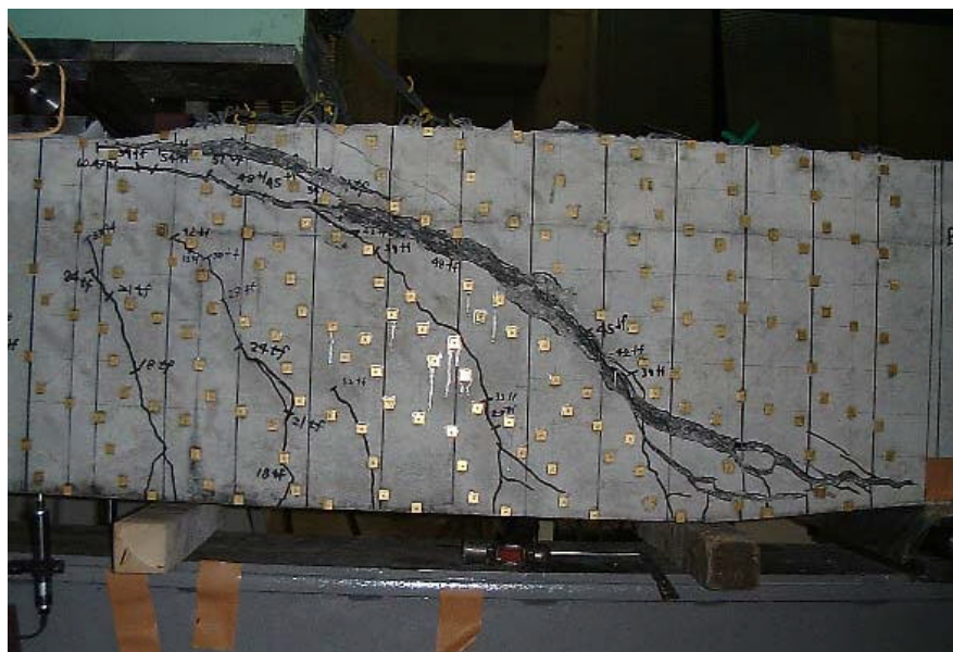
Figure.3_2: Shear failure of Beam 1.
