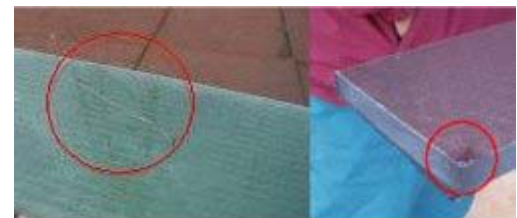
Fig.2 Damages after Artificial Thunder Striked. (Left) GFRP (Right) CRP
