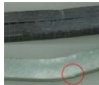
Fig.4 Destructive Mode of GFRP and CFRP
