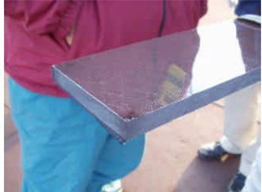
Fig.2 Lightning Damage in CFRP
