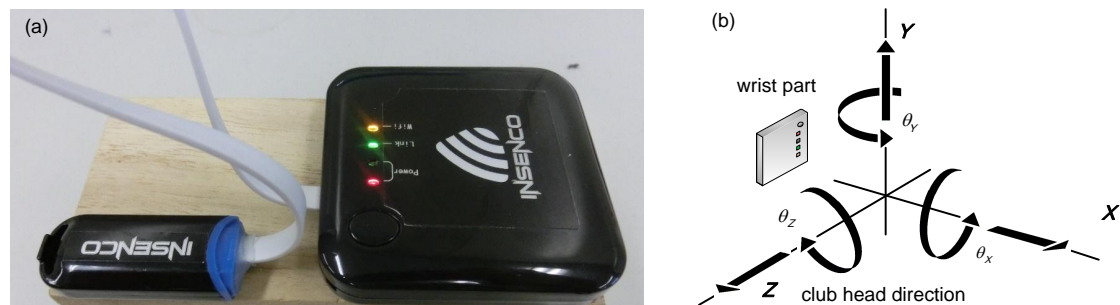
Figure 6.4 – Motion sensor for golf swing. (a) motion sensor; (b) definition of coordinate system.
