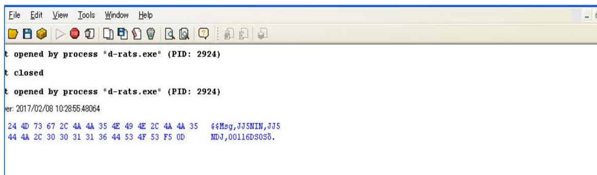
Figure 4.16 SOS message raw data received by the serial monitoring software.
