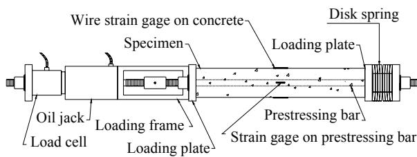
Fig.3.4.3: Testing apparatus
