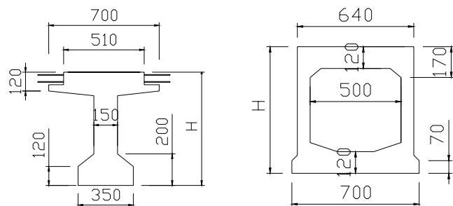
Fig.3.2.2: Dimensions of T-shape and box shape girders
