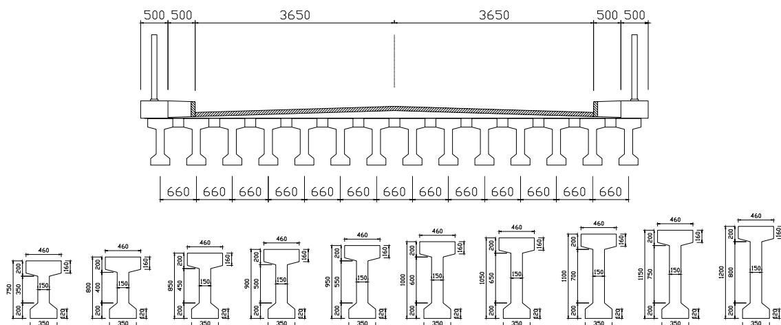
Fig.3.2.5a: Typical two lanes girder bridge of T-shape with heavy bottom flange (14 girders)
