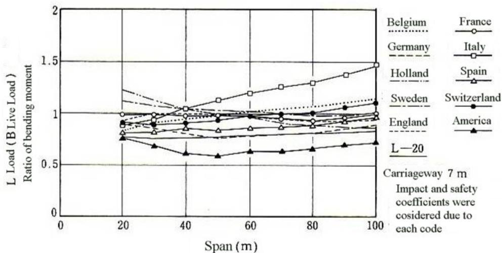
Fig.3.1.1.3: Comparison of bending moment between various codes
