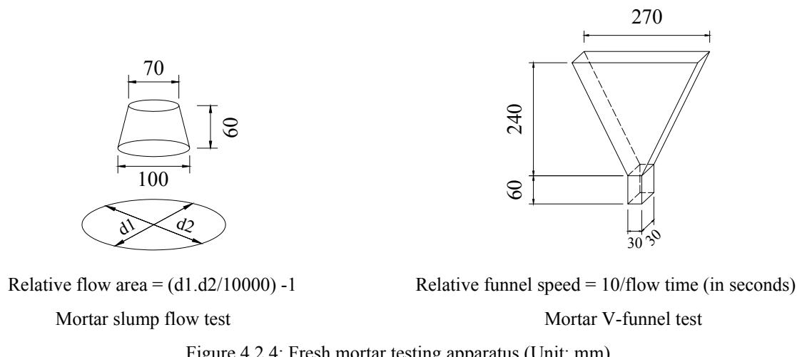
Figure 4.2.4: Fresh mortar testing apparatus (Unit: mm)
