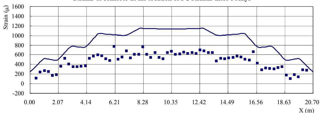
Fig.5.4.1: Strains of concrete at the location of PC strands
