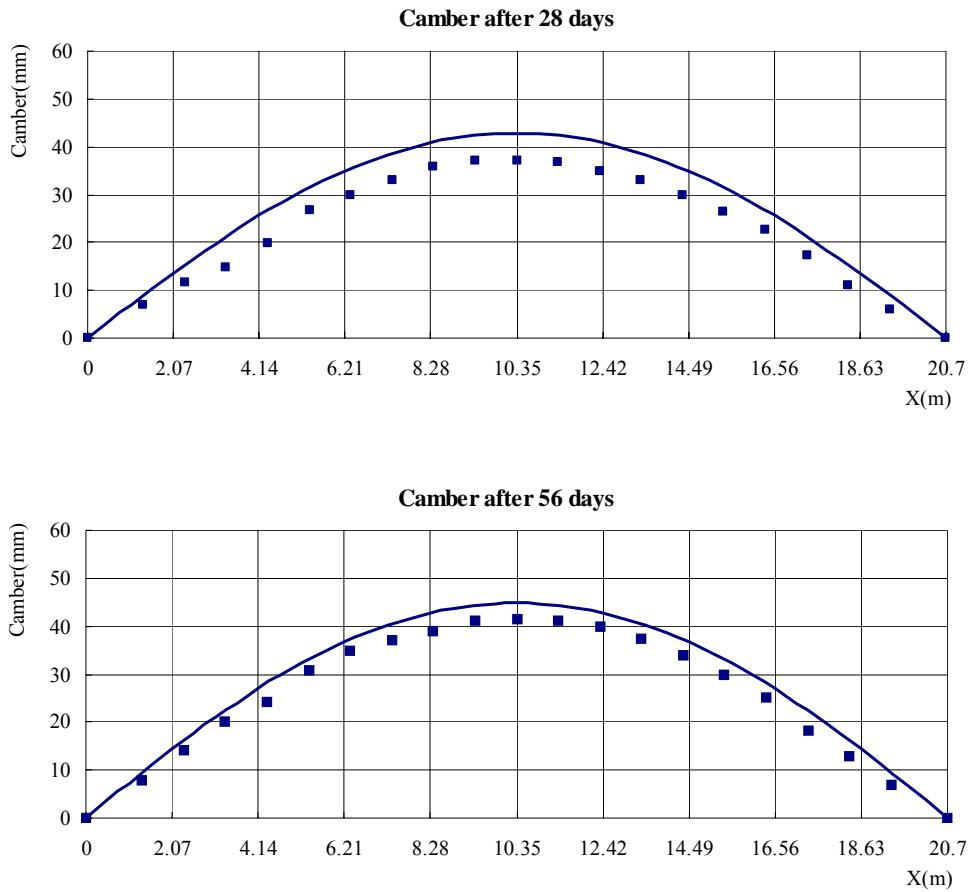
Fig.5.4.3: Time dependent camber along the PC girder
