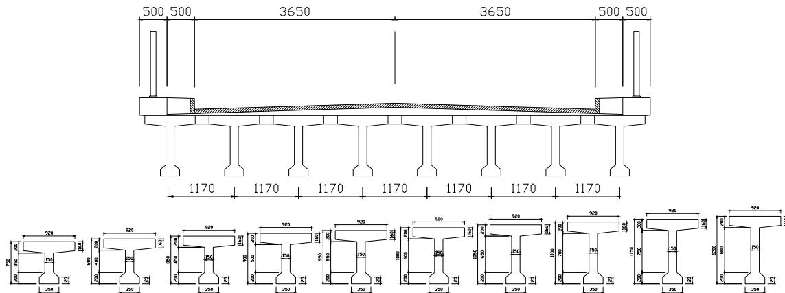
Fig.3.2.5b: Typical two lanes girder bridge of T-shape with heavy bottom flange (8 girders)
