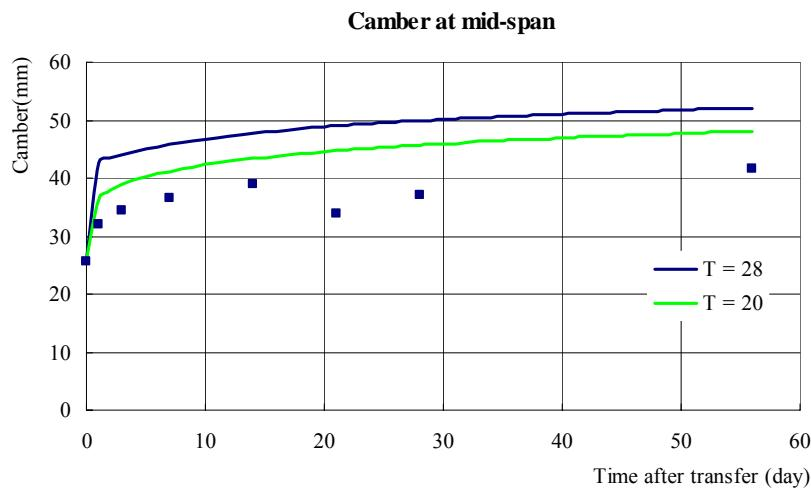
Fig.5.4.10: Camber at mid-span by using CEB-FIP90 code
