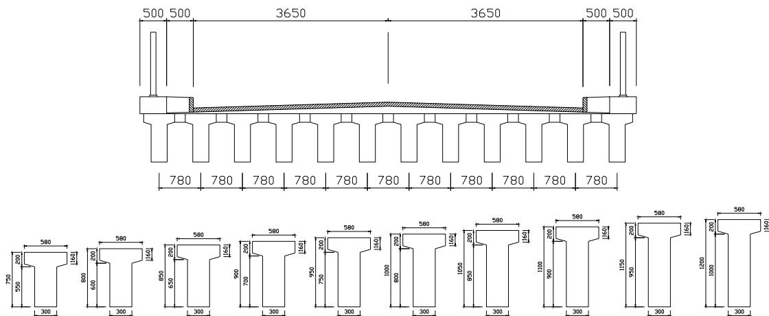
Fig.3.2.4: Typical two lanes girder bridge of T-shape
