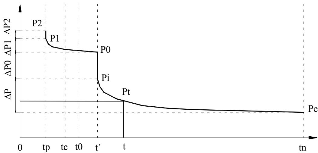
Fig.3.5.2.1: Process of prestress loss in pretension system
