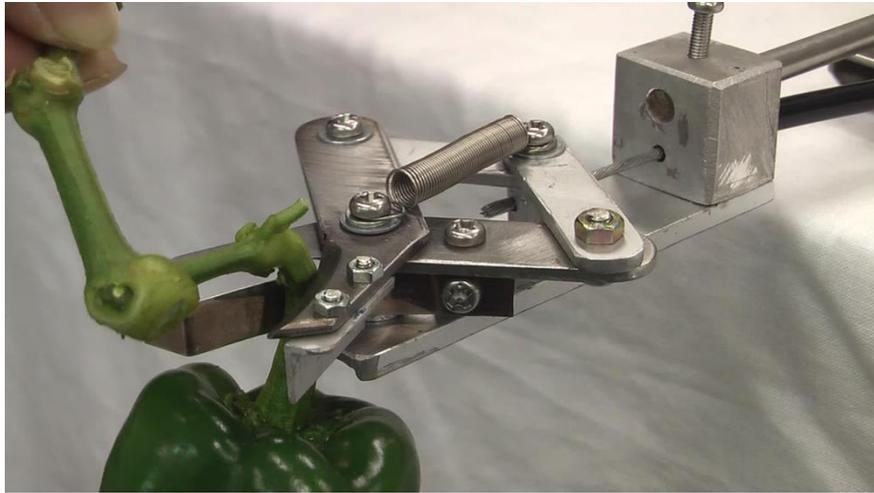
*Figure 4-7* The end-effector used by the harvesting robot.
