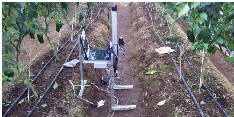
*Figure 3-2* Pose estimation setup for the greenhouse test
