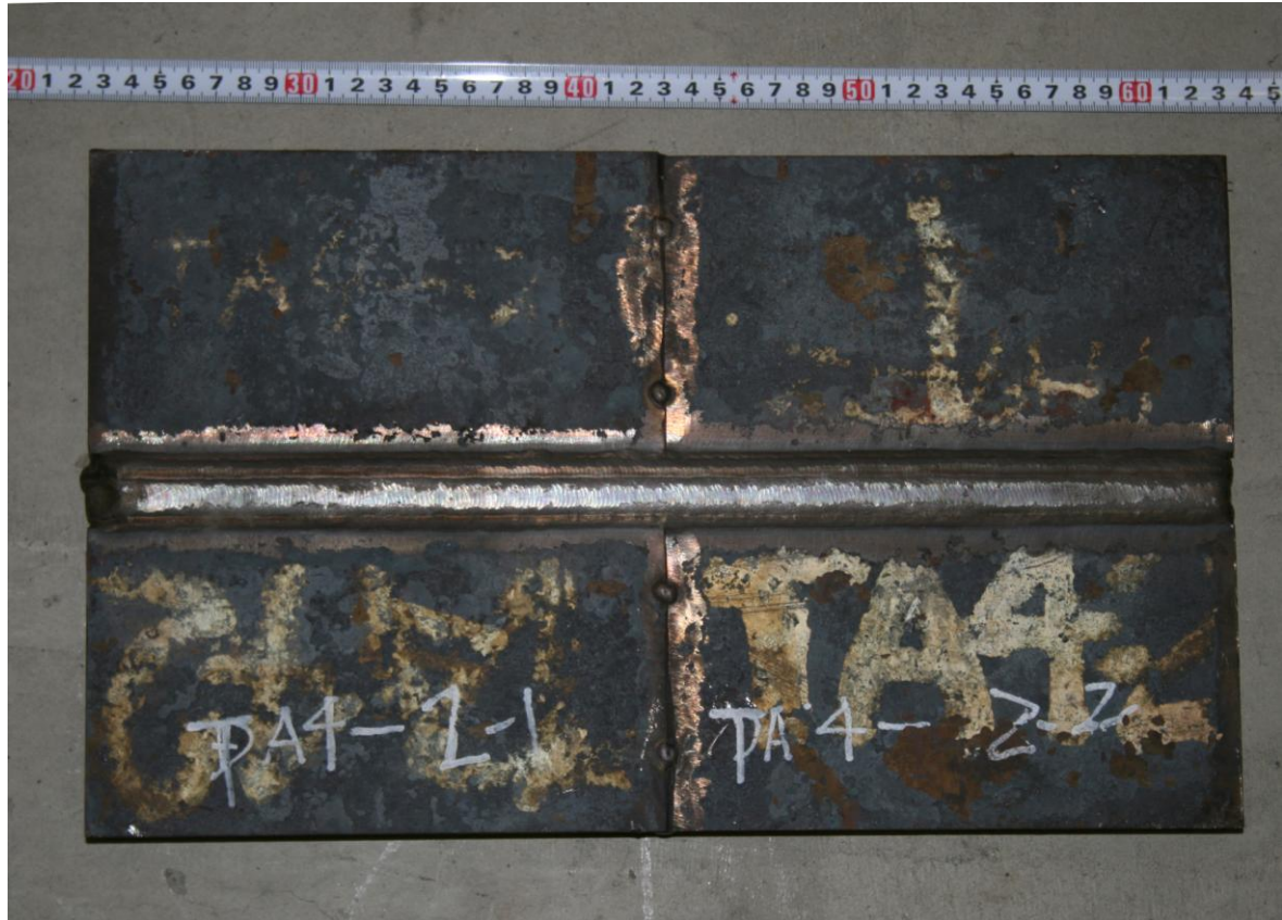
Fig. 2-1. As received GTAW joint of Mod.9Cr-1Mo steel plate with 25mm thickness.
