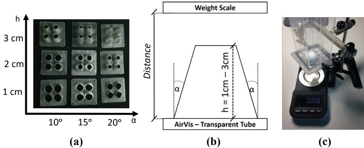
Figure 3.3: Nozzle effect test, (a) various nozzle with different height and angle, (b) illustration of nozzle dimension with  $h =$  nozzle height and  $\alpha =$  nozzle angle, and (c) air flow force measurement setup (AirVis is put upside down and perpendicular to digital scale, with changeable distance).
