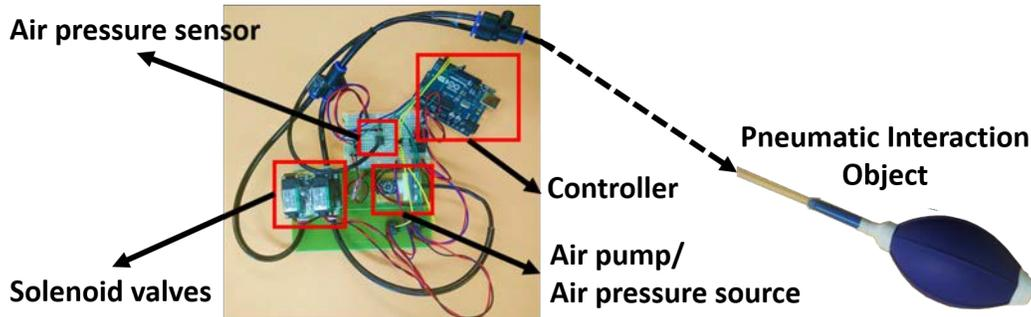
Figure 4.8: Complete Pneumatic System.
