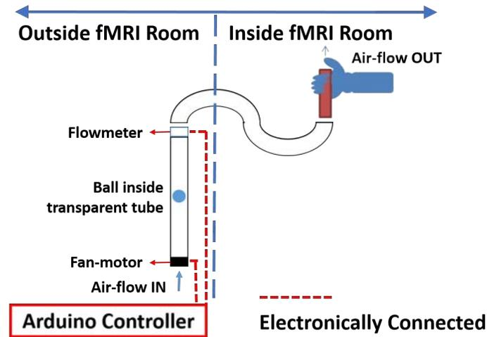
Figure 4.3: Schematic diagram of air-flow based system.
