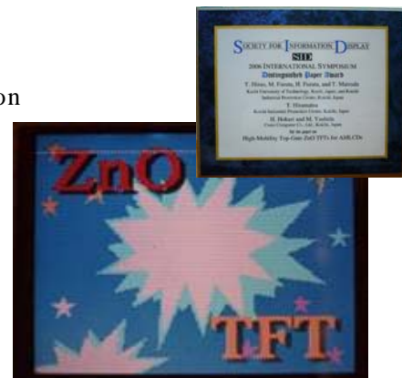
Photo: LCD panel driven by ZnO TFTs
