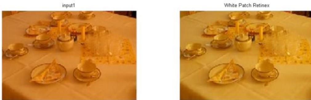
**Figure 1. 34** The white patch retinex algorithm is used to perform the color adjustments for the input image, the result is show in the right side. From Ebner(2007).
