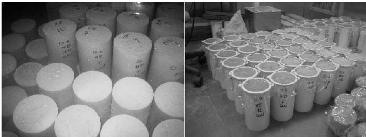
Fig III.3-1: Curing methods: wet curing and seal curing
