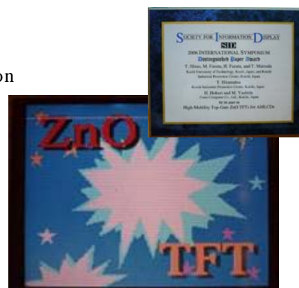
Photo: LCD panel driven by ZnO TFTs
