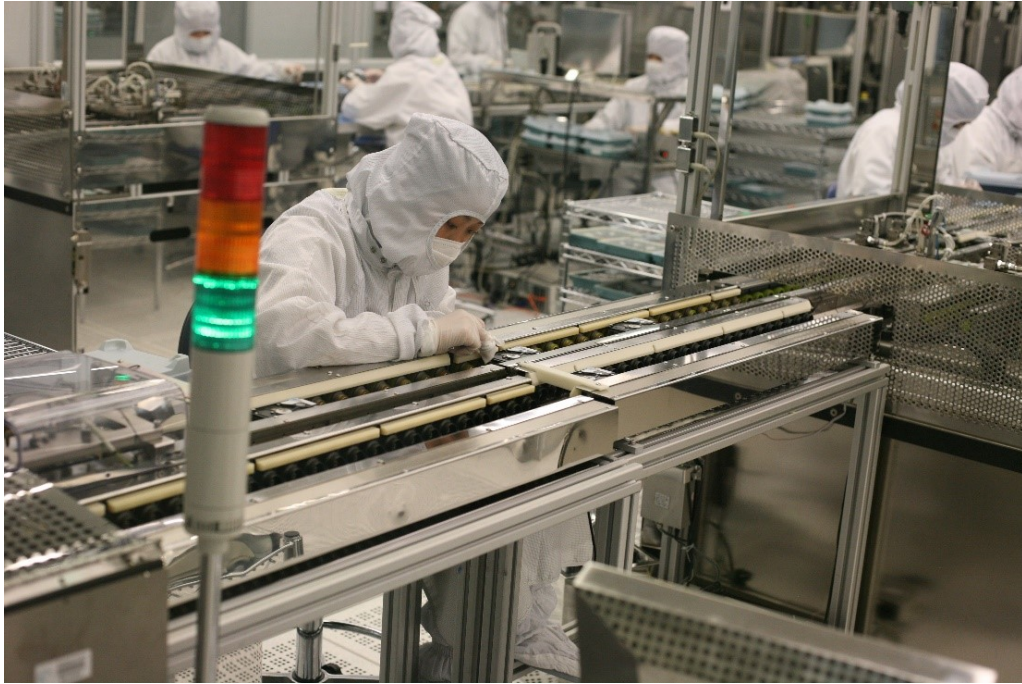
Figure 1.1: Hard disk assembly in a Seagate clean room. 2
