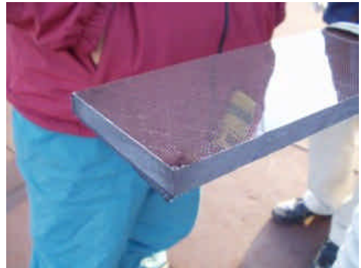
Fig.2 Lightning Damage in CFRP
