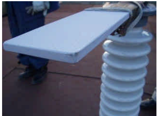
Fig.3 Lightning Damage in Aluminum Coated GFRP
