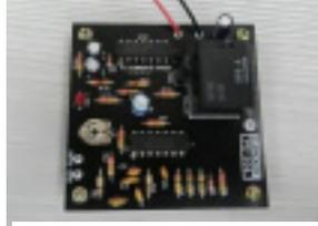
Fig2. Touch sensor with sensor relay
