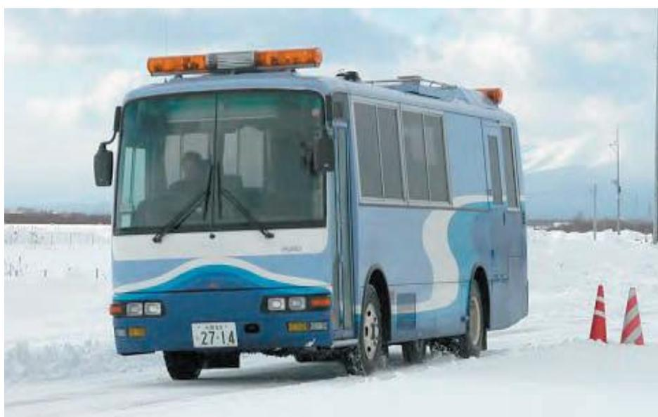
Fig.1-1 Slip measurement vehicle
