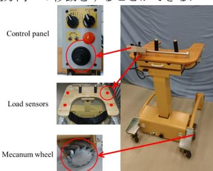
Fig. 1 Intelligent walking support machine.
