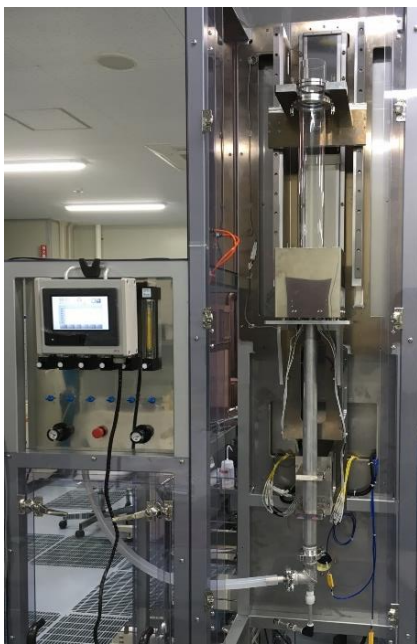
Fig.6 4generational mist CVD system
