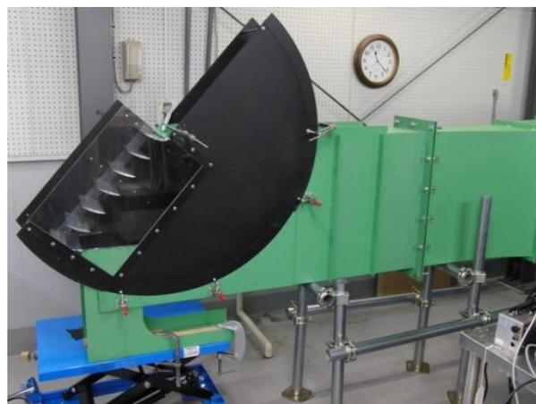
Fig.2 Linear cascade wind tunnel
