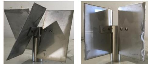
Fig.7 Slant paddle(left) and vertical paddle(right)
