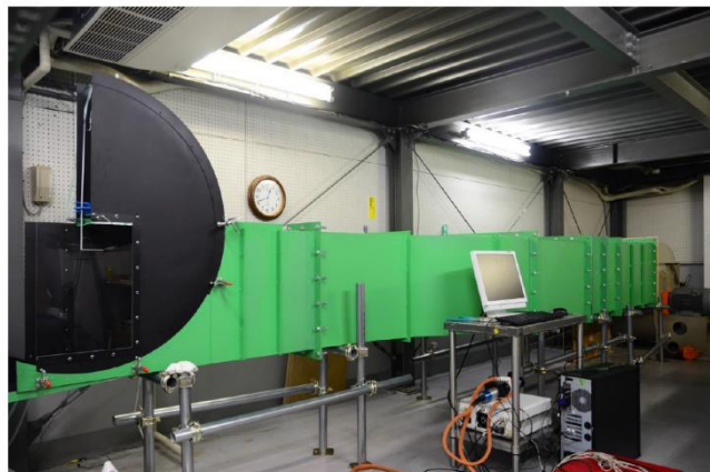
Fig 1 Linear cascade wind tunnel
