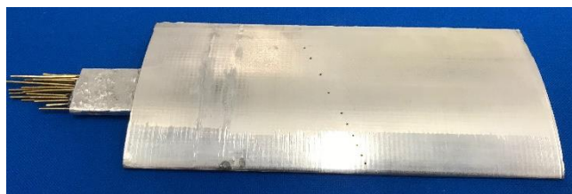
Fig 3 static pressure measurement vane
