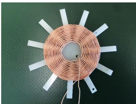
Fig.9  $\phi=0.08\text{mm}$  30 twisted ritz wire coils
