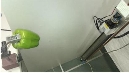
Fig.9 Recognition of peppers of camera and laser range finder by slider movement
