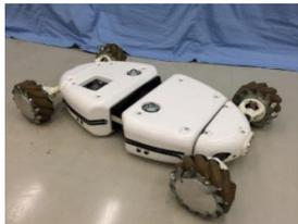
Fig.1 Non-direction Four-wheeled Mobile Robot
