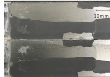
Fig.7 Fracture surface of specimen with dripping 30 day (60°C)
