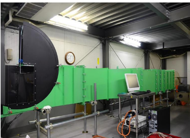
Fig. 1 Linear cascade wind tunnel.
