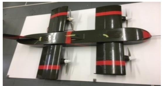
Fig.1 prototype of QTW aircraft
