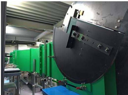
Fig. 1 Cascade wind tunnel.
