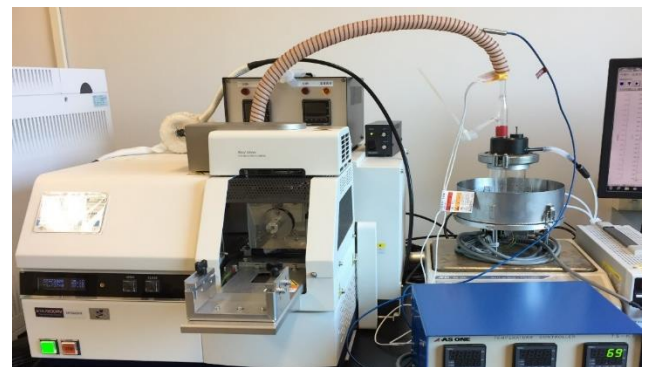
Fig. 2 Reaction field atmosphere control corresponding TG-DTA system
