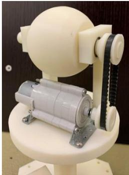
Fig. 3 Power transmission mechanism (Left).
