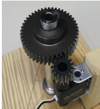
Fig. 4 Direction determination mechanism (Right).
