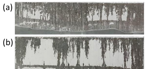
(a) polished specimen (b) plasma etched specimen Fig.6 Fracture surface of specimen.
