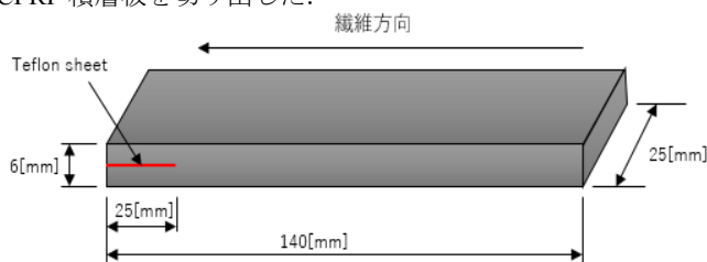
Fig.1 Dimensions of DCB specimen
