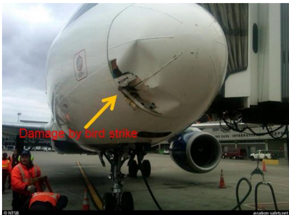
Fig.4 Damage on forward pressure bulkhead
