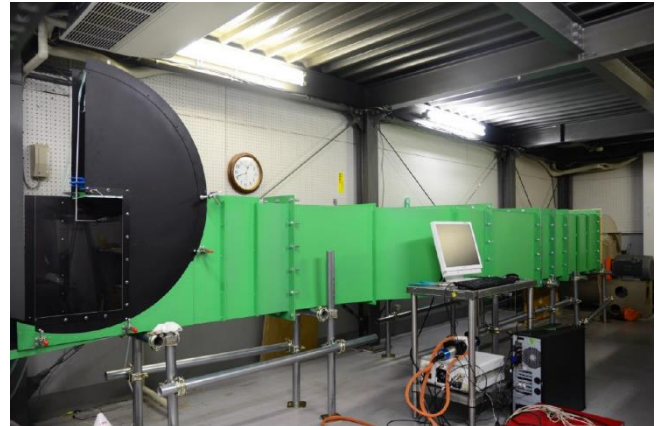
Fig. 1 Linear cascade wind tunnel
