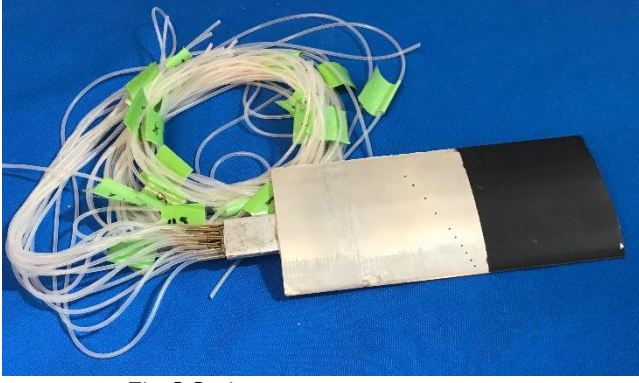
Fig. 3 Static pressure measurement vane
