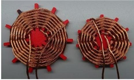
Fig.13 Transmission coil (left) and receiving coil (right)
