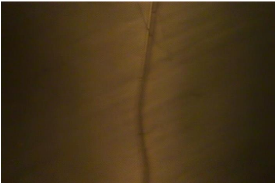
Fig. 1 Polarized light microscopic image of a nematic liquid crystal under shear flow between the concentric cylinders
