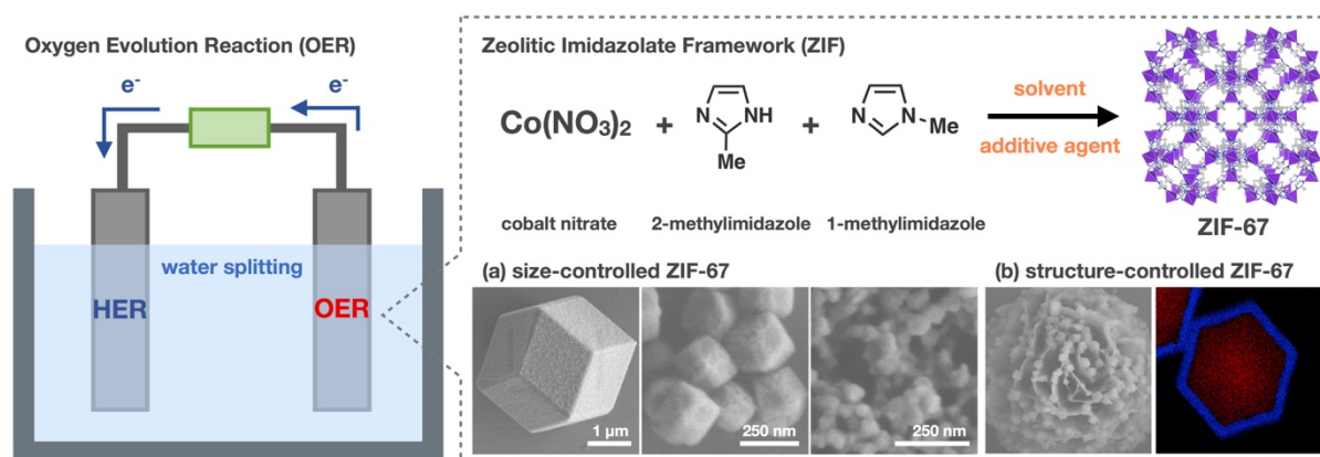
Figure 1. (left) Schematic illustration of water splitting. (right) Scheme, SEM and overlaid EDX mapping images of size- and structure-controlled ZIF-67.
