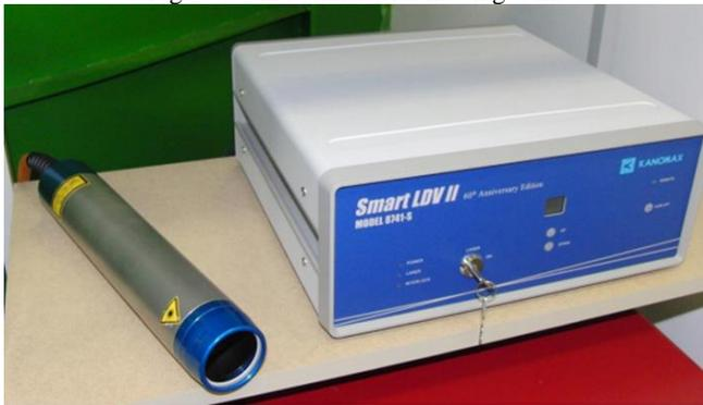
Fig. 4 Laser Doppler velocimetry.
