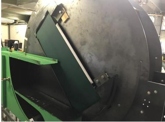
Fig. 3 Wind tunnel with moving wall.
