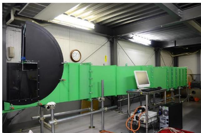
Fig. 1 Linear cascade wind tunnel.
