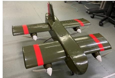
Fig. 1 QTW aircraft for experiment
