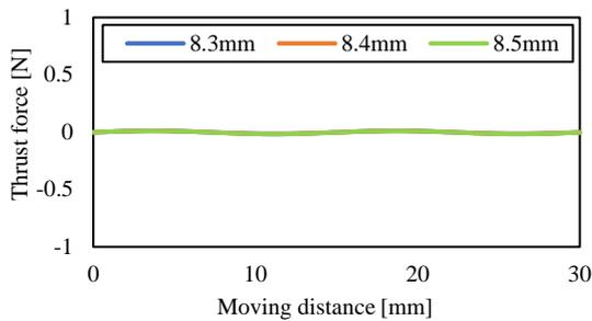
Fig.2 Thrust force when moving horizontally at each air gap
