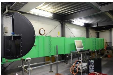
Fig. 1 Linear cascade wind tunnel.
