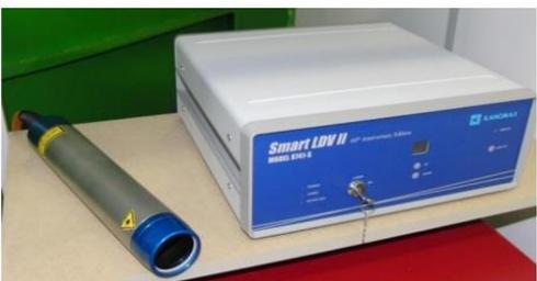
Fig. 7 Laser Doppler Velocimeter.
