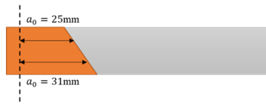
Fig.3 GFRP specimen (Top view)
