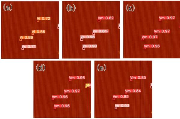
Fig. 3 Typical examples showing automatic detections of three types of vacancies on InP(110)-(1x1) surfaces, using models trained by augmented data set. (a) aspect ratio conversion. (b) rotation. (c) translation. (d) flip. (e) shear deformation.  $V_m$ ,  $V_s$ , and  $V_i$  indicate monovacancy, vacancy string and vacancy island, respectively.
