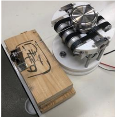
Fig.4 Experiments to measure the maximum static friction coefficient
