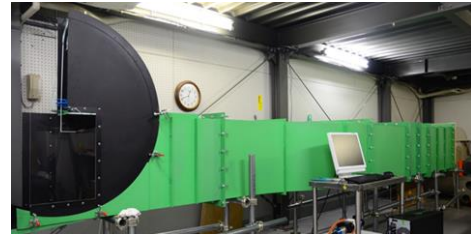
Fig. 2 Linear cascade wind tunnel.
